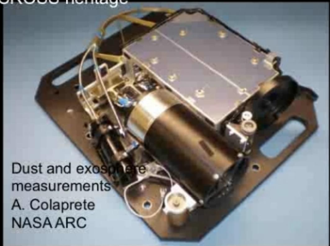
UVS is a spectrometer, not an imager, and so we need to identify dust based on its spectral properties
