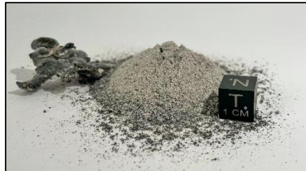
Figure 2. Agglutinated LHS-1 Simulant and large agglutinate
