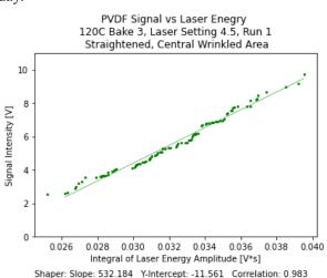
Figure 1: Laser pulse strikes on PVDF and linear fit after the film was exposed to 7 days cumulatively at 120C.
