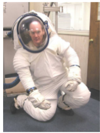
I-Suit with a modified DuPont Tyvek® cover garment in first order interface test
